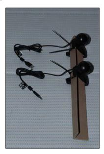
A closer and frontal view shows the camera lenses, which can be regulated manually in focus. Note that you should set it to some appropriate distance (1 to 2 meters used for the baseline should be good in the most general case):
