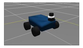
The system had to know the position of the new laser to detect collisions, such as the one between wheels and walls. With the TF tree, this is very simple to do and maintain and is also scalable. Thanks to tf, we can add more sensors and parts, and the tf library will handle all the relations for us. All the sensors and joints must be correctly configured on tf to permit the navigation stack to move the robot without problems, and to exactly know where each one of their components is.
