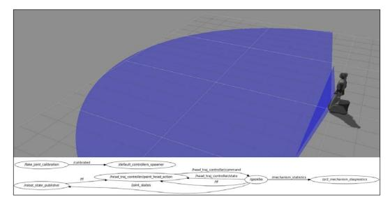
In the screenshot you can observe REEM has two frontal range lasers. One pointing forward with a large range and another slightly tilted down. We could load any environment we want in Gazebo and use the navigation stack to make the robot move through the simulated environment, as discussed in previous chapters.
