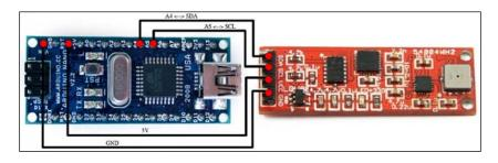
The only thing necessary is to connect the four wires to make it work. Connect the **GND** and **Vcc** from the sensor to **GND** and **5** V in Arduino.
