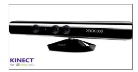
In ROS, we are going to use two of these sensors: the RGB camera and the depth sensor. In the latest version of ROS, you can even use three.
