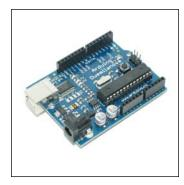
ROS can use this type of device with the package rosserial. Basically, Arduino is connected to the computer using a serial connection and data is transmitted using this port. With rosserial, you can also use a lot of devices controlled by a serial connection; for example, GPS, servo controllers, and so on.
