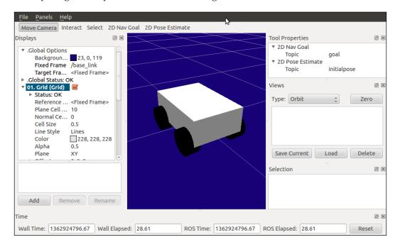
Let's finish the design by adding some parts: a base arm, an articulated arm, and a gripper. Try to finish the design yourself; you can find the final model in the chapter5\_tutorials/urdf/robot1.urdf file. You can see the final design in the following screenshot as well:
