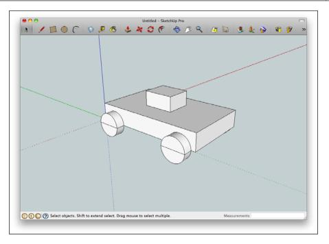
The model was exported only to one file, so the wheels and chassis are the same object. If you want to make a robot model with mobile parts, you must export each part in a separate file.
