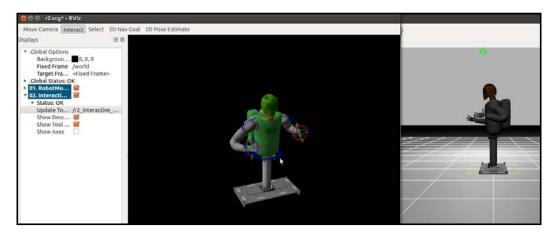
We observe the interactive markers that we can control directly in rviz, which allow us to give the desired position of the hands, and by inverse kinematics of the arm chain the joint's state is obtained so the arm reaches the desired pose.
