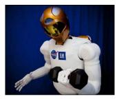
The R2 shown in the previous picture was launched to the International Space Station (ISS) as part of the STS-133 mission, and it is the first robot of its kind in space. It is important to note that R2 is deployed on a fixed pedestal inside the ISS, as we will see in the simulation environments in the sequel. However, other robonauts will be attached to a four-wheeled vehicle, or will have legs in the future.
