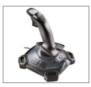
In ROS, a joystick is used to telecontrol a robot for changing its velocity or direction.
